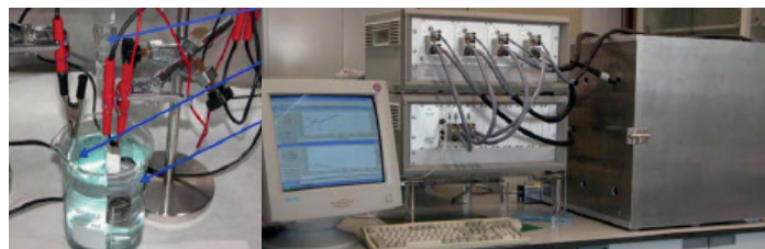
Figure 2: Bench for electrochemical testing
